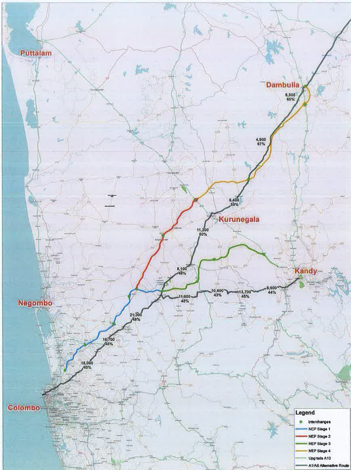
Figure 3-3: Average Weekday Daily Traffic Flow on A1 and A6 (Cars and Commercial Vehicles) - % = commercial vehicles
